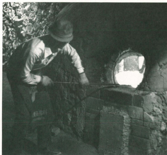
Firing the kiln, 1872. Starting at the bottom, each chamber has been fired separately to temperature and sealed. The stoker visible in this sketch is working in tandem with another man on the other side of the kiln. A child fans the flames away from the man's face. Illustrations from Shigaraki-yaki Zukai , manuscript owned by the Shiga Prefectural Library, Otsu, Japan. Photos by Louise Cort, Smithsonian Institution
