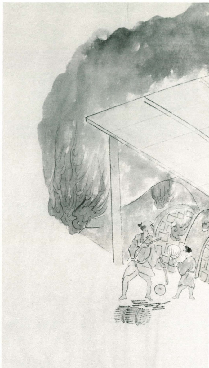
Firing the kiln, 1872. Starting at the bottom, each chamber has been fired separately to temperature and sealed. The stoker visible in this sketch is working in tandem with another man on the other side of the kiln. A child fans the flames away from the man's face. Illustrations from Shigaraki-yaki Zukai , manuscript owned by the Shiga Prefectural Library, Otsu, Japan. Photos by Louise Cort, Smithsonian Institution
