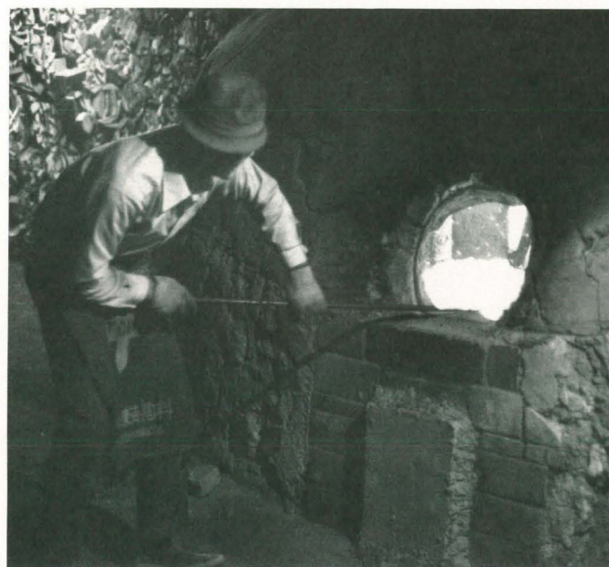
Firing the kiln, 1872. Starting at the bottom, each chamber has been fired separately to temperature and sealed. The stoker visible in this sketch is working in tandem with another man on the other side of the kiln. A child fans the flames away from the man's face. Illustrations from Shigaraki-yaki Zukai , manuscript owned by the Shiga Prefectural Library, Otsu, Japan. Photos by Louise Cort, Smithsonian Institution
