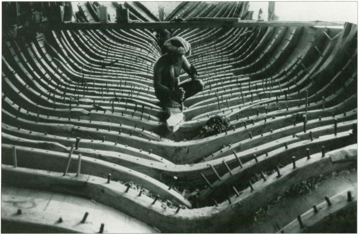
Above: Sulawesi boatbuilders are renown throughout Indonesia. This boatbuilder near Majene, South Sulawesi, works with simple tools. The dowels are made of ironwood and the caulk of crushed coral and oil. The large ship he is building will carry cattle and passengers between Kalimantan (Borneo) and Sulawesi. Photo by Charles Zerner
