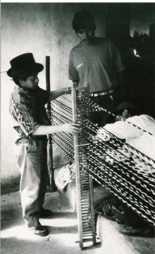
Francisco Sic and Jaime Walter Garcia string an exact number of resist-dyed threads for a loom warp to create a desired textile pattern. CDRO's most profitable project, the Programa Artesanal annually ships textiles worth $100,000 from Totonicapán to markets throughout the world. Photo by Nestor Vega
