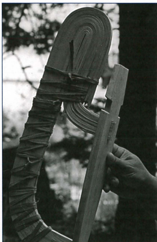
Fig. 3. Canoe-prow assembly with "man-board" — so called because it resembles a human form. A single piece of cedar is used which is split into more than 30 laminations to effect the bends in its form. These are held in place using wiigoob (the inner bark of the basswood tree) and threaded through and inserted over the man-board. Photo by Janet Cardle
