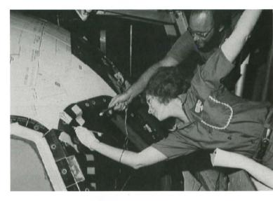
Technician Pat Klose leans over an edge in order to repair one of the protective thermal tiles on the Space Shuttle *Columbia*, prior to its fourth launch in 1982.
