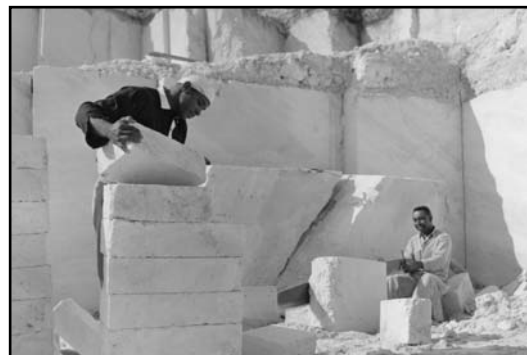
Top: Cutting limestone blocks.
