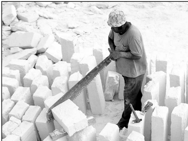
Top: Cutting limestone blocks.
