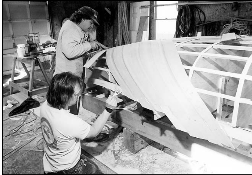
Building a Bermuda fitted dinghy using composite strip molding method. Courtesy Royal Hamilton Amateur Dinghy Club.
